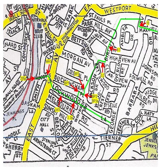
Figure 16 Detail of drainage pipe system between Buckingham Place and Lockwood Lane. The flow of contaminated water goes south past Site BP2 to Site BP3/BP3a. Water flowing to the west at Site BP3a is only mildly polluted (small pipe of unknown origin). The combined stream flows west to Site BP1 and then south to Site3/3a on Lockwood Lane where it joins the Lockwood drainage pipe.
