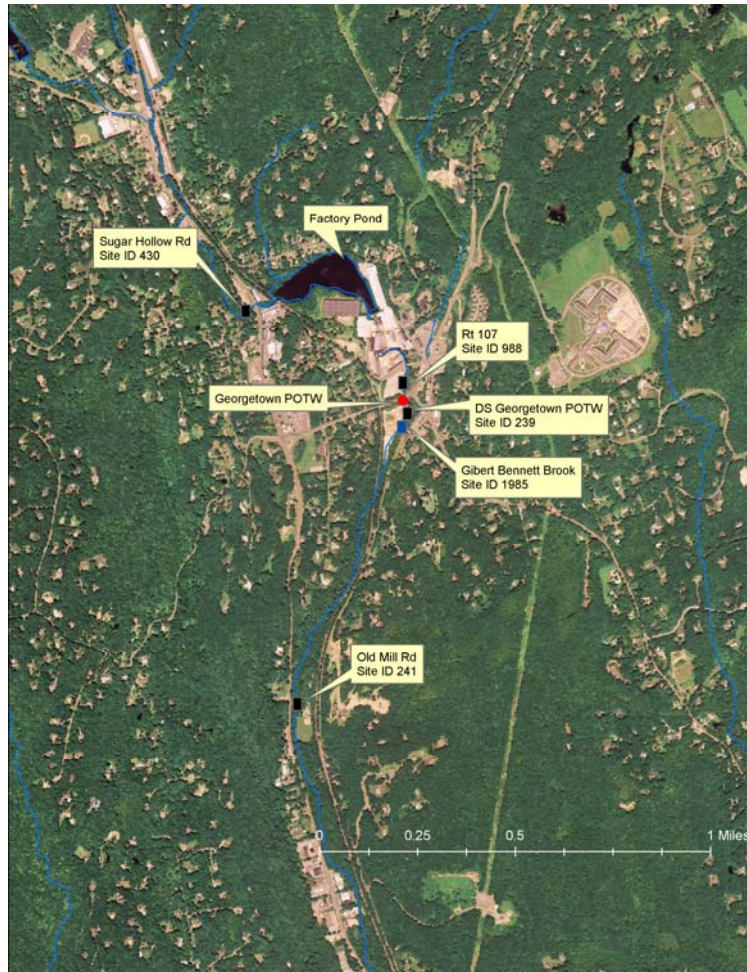
Figure 9. Map showing locations of monitoring locations in the Georgetown section of the Norwalk River. Monitoring sites are shown as black squares, the Georgetown sewage treatment plant is shown as a red circle , and tributaries are shown as a blue square .
